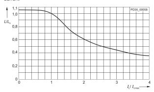
Typical curve of the inductance of a **commutating reactor** over the reactor current
