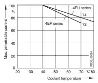
Deviation of the permissible direct current of rated direct current  $I_{\rm dn}$ , or permissible alternating current of rated alternating current  $I_{\rm n}$  (at coolant temperatures  $\neq$  40°C)
