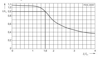
Typical curve of the inductance of a **mains reactor** over the reactor current
