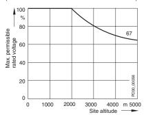
Reduction of rated voltage for insulation (at site altitudes > 2000 m above sea level)
