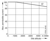
Deviation of permissible direct current of rated direct current  $I_{\rm dn}$ , or permissible alternating current of rated alternating current  $I_{\rm n}$  (at site altitudes > 1000 m above sea level)
