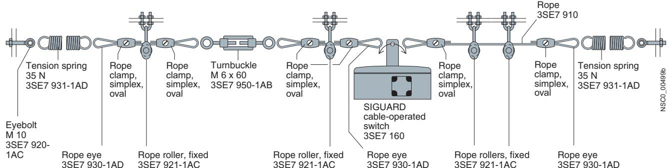
Use of a tension spring is essential for long sections of rope.
