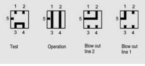
Fig. 1/77 Cock positions; the symbols are printed on the cock
